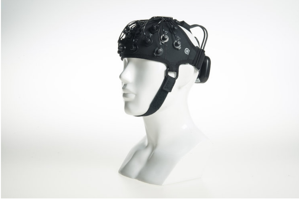
Figure 2.3: Portable Bluetooth fNIRS device (Brite from Artinis) ( Source: artinis.com ).
